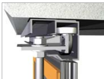
Laufschienenprofil in Laibung - running rail profile – in embrasure
